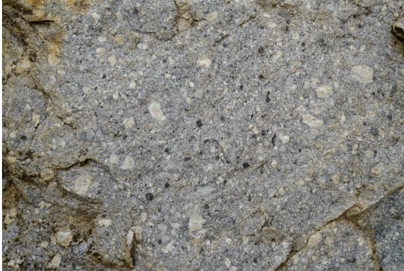
Figure 21.- Cordierite-garnet granite. The large green spots are cordierite-garnet aggregates. This rock appears as a large NW-SE dike in the middle eastern part of the batholith.
